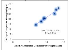
Figure 1.5: Simple Linear Regression relationship for RAC 100 % Replacement (28-Days)
