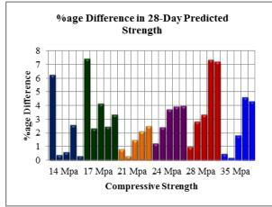
Figure 1.6 (a): %age difference in Predicted Compressive Strength (28-Days), (compressive strength as basic parameter)
