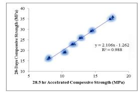
Figure 1.1 : Simple Linear Regression relationship for control mix 0 % Replacement (28-Days)
