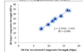
Figure 1.2 : Simple Linear Regression relationship for RAC 25 % Replacement (28-Days)
