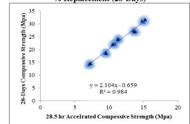
Figure 1.3 : Simple Linear Regression relationship for RAC 50 % Replacement (28-Days)
