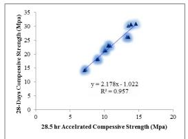
Figure 1.4 : Simple Linear Regression relationship for RAC 75 % Replacement (28-Days)
